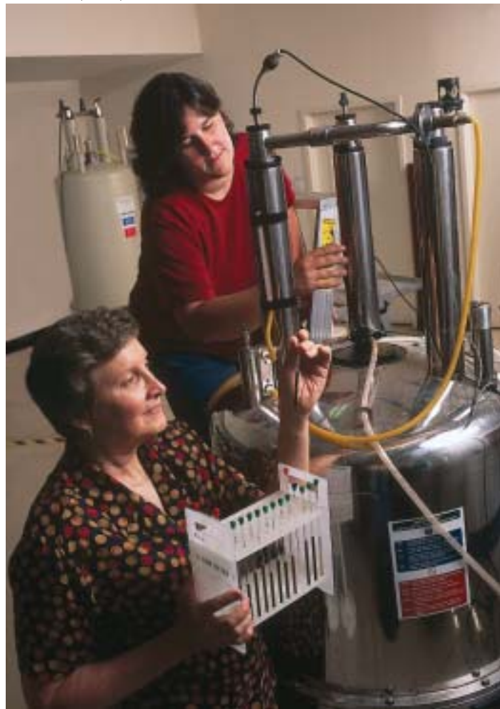
Sara Wright (foreground) and technician Kristine Nichols use nuclear magnetic resonance to examine the molecular structure of extracted soil organic matter constituents.
